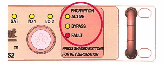
The following steps configure a new or zeroized LinkWays2 modem for encryption using the modem's front panel controls and LCD. Note that a new or zeroized LinkWay 52 modem will have no traffic keys, the Active LED will be flashing green, and the Fault LED will be flashing red.
